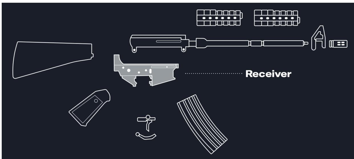
58. Most ghost guns are made from “unfinished” frames and receivers—meaning frames and receivers that are “solid” and lacking in machine marking or drilling in certain specified areas (typically the fire control cavity or trigger area). Unfinished frames and receivers are often
